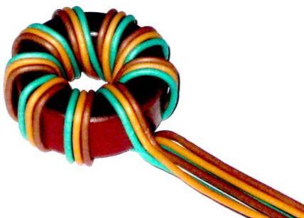
1. A trifilar winding is used. Cut 50 cm lengths of different colored insulated wire of at least 0,75 mm<sup>2</sup> cross section. As you can see in the photo I used red, yellow and green wire. [multi stranded wire from a discarded computer power supply should work well.] Use about 9 windings (one winding on a toroid is counted each time a conductor passes through the centre hole). Details of the toroid core are given below.
